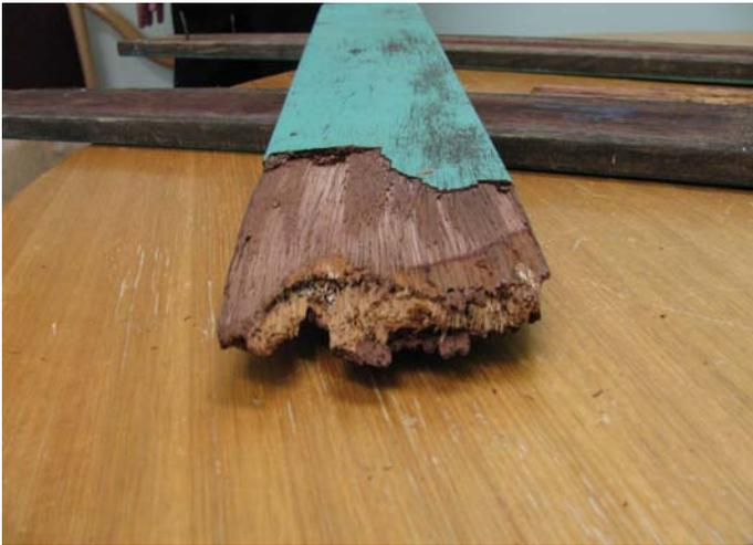
**One of the decayed decking boards from the 2010 accident.**
